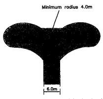
An acceptable irregular shaped turning head must be able to accommodate a standard turning head
