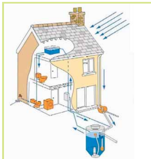
Rainwater collection and reuse system © Environment Agency
